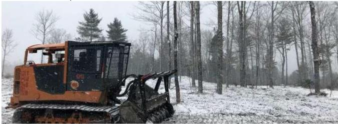
A forestry mulcher machine shown here may be used for trail and woodcock singing field establishment. It does not remove stumps; it grinds them into the soil so the site may be mowed by a tractor. Can also be used to grind slash left behind after a timber harvest to mitigate aesthetic concerns and may be used for tree planting site prep.
